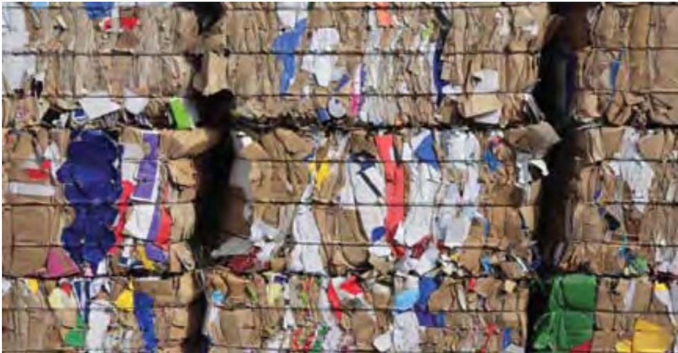
Recycled paper and old cardboard container paper is fully saturated with a pigmented PetroFree™ resin, then dried to a "B" stage paper (tacky but not sticky). Because of the natural characteristics of recycled paper, not all saturation levels are the same across the sheet. Unlike virgin fiber, this *flocculation* is what gives PaperStone® its unique, mottled look. Both the mottling and speckling of PaperStone® are enhanced by sanding away the surface micro-textured resin layer.
