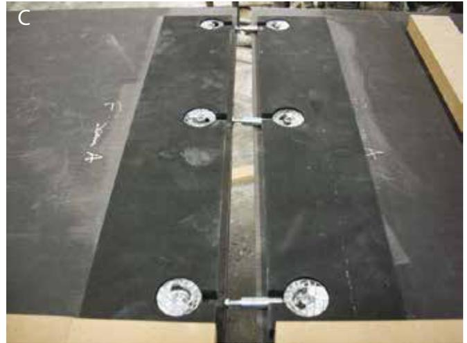
This seaming system (see fig. A-B-C-D) can be used on kitchen worktops with a thickness of 19mm, using elements such as Maxifix 35, which is produced by the company Hafele ([www.hafele.com](http://www.hafele.com)).
